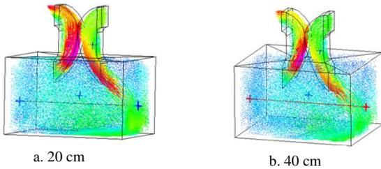
Figure 8. Flow patterns for different bottom lengths of two-canal centred position windcatchers
