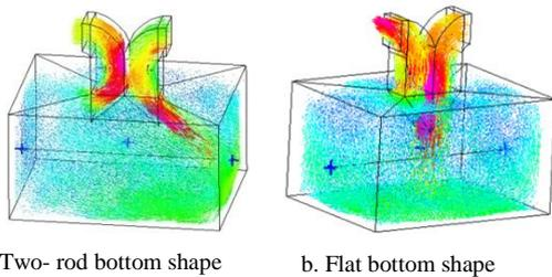
Figure 5. Flow patterns for centred position windcatchers with different bottom shapes
