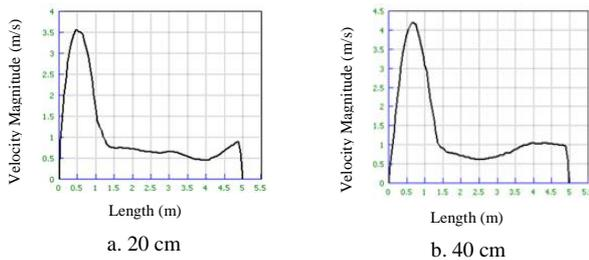
Figure 9. Velocity magnitude for different bottom lengths velocity of two-canal centred position windcatchers
