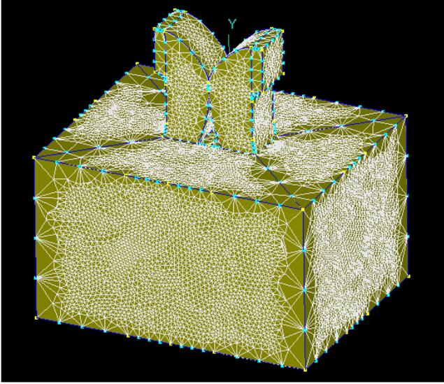
Figure 2. Unstructured triangle meshes in a model
