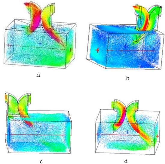
Figure 3. Flow pattern for different windcatcher's positions with inlet velocity of  $3 \text{ m/s}$
