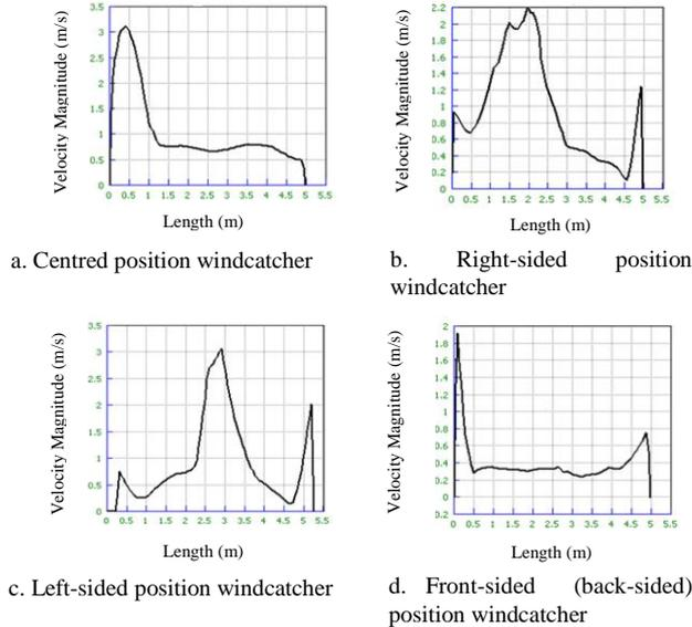
Figure 4. Velocity magnitude along the room at level 1.2m above the floor for different windcatcher's positions
