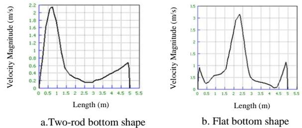
Figure 6. Velocity magnitude along the room at level 1.2m above the floor for centred position windcatchers with different bottom shapes
