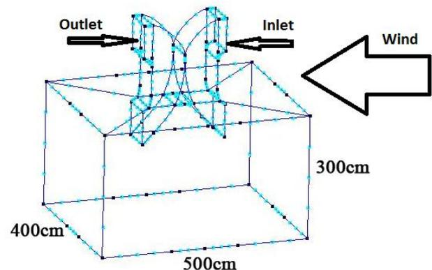
Figure 1. A modelled room fitted with a windcatcher
