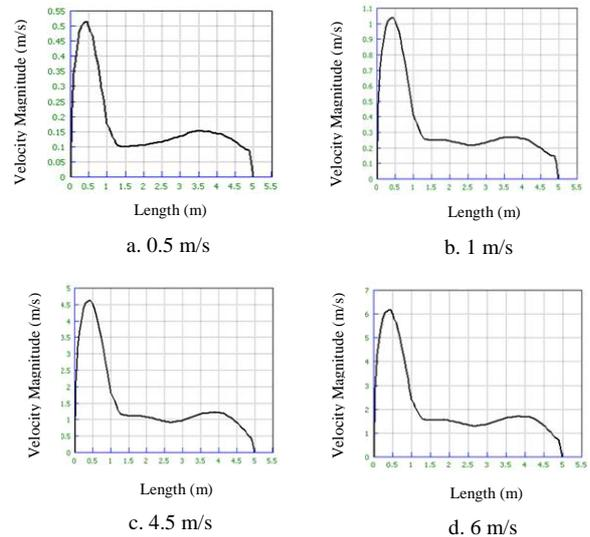
Figure 7. Velocity magnitude along the room at level 1.2m above the floor for centred position two-canal windcatcher with different inlet velocities
